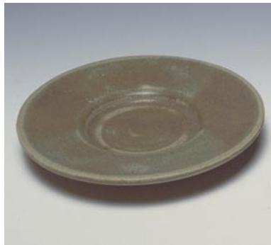
Figure 2-1. Toshika Green is a beautiful matte green glaze; however, as you see in Figures 2-2 and 2-3 it should only be used for decorative work. It is not sufficiently durable for functional pottery.
