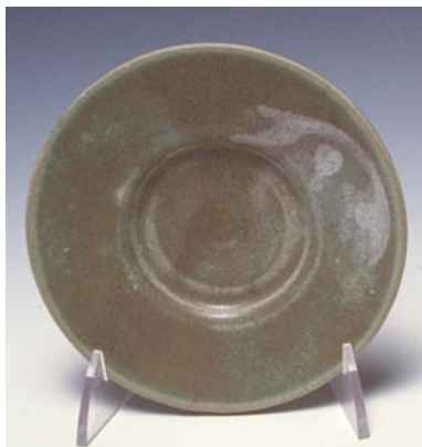
Figure 2-2 (left). A juicy slice of lemon was placed on the sample for 2 hours at room temperature.
