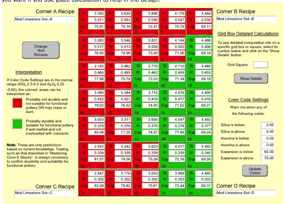
Figure 5-6. By modifying a standard grid in the way described you can significantly increase the area of interest for functional glazes.
